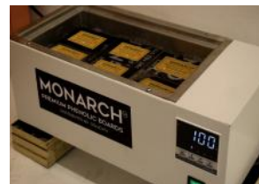
8-Hour Boil Test
