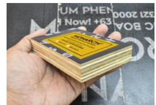
Superior Bonding Quality (After boil test)
